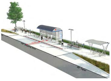
Figure 72. Shelters, lighting, seating, bike racks, and greenscaping are important components of transit stops that promote well-being. Image Credit: Reimagine Washtenaw
