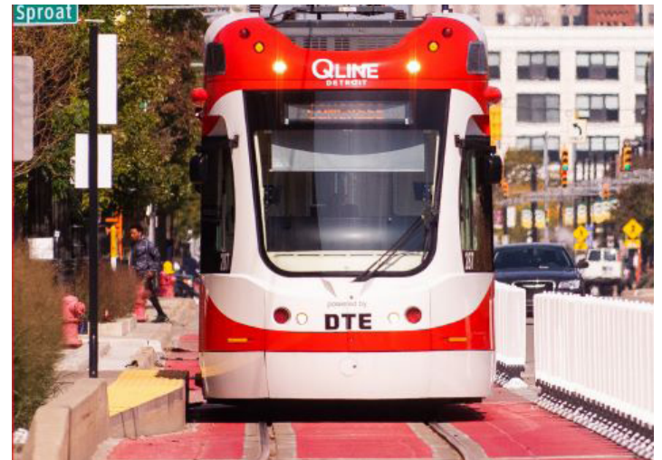
Figure 34: The dedicated transit lane on Woodward Avenue allows QLINE, DDOT, and SMART to avoid congestion near Little Caesar's Arena. Image Credit: M-1 RAIL.
