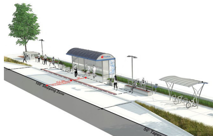
Figure 39: Shelters, lighting, seating, bike racks, and greenscaping are important components of transit stops that promote well-being. Image Credit: Reimagine Washtenaw.
